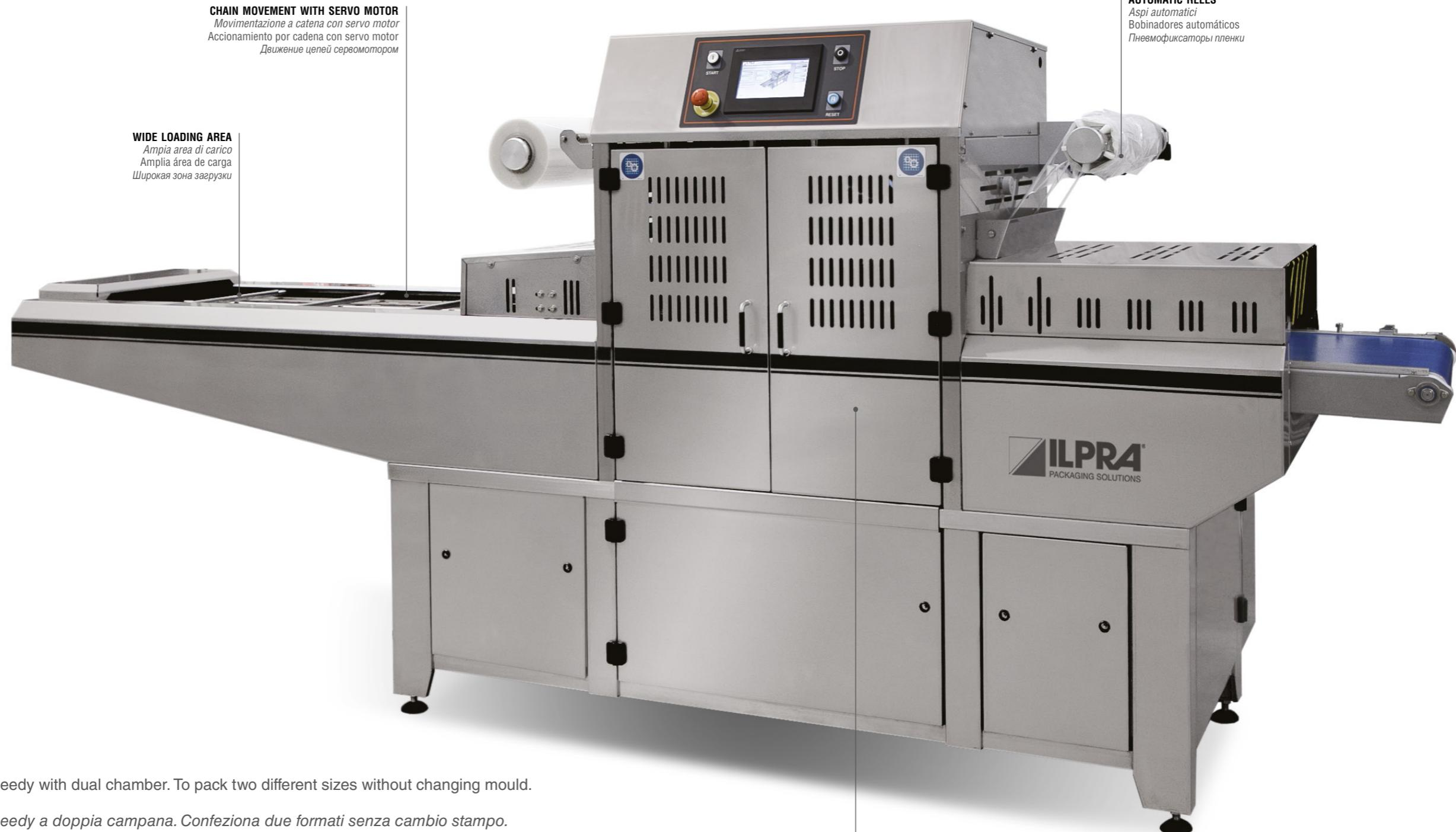
FoodPack SPEEDY DUO: speedy with dual chamber. To pack two different sizes without changing mould.
